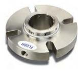
Premium-grade construction is standard, with options for FFKM or EPR elastomers and premium carbon, sintered silicon carbide faces. The FSI Series 1015 features viton elastomers, 316 stainless steel hardware. and a large flush port for API plan 11, 13, or 32 operation. Its self-aligning stationary design features a flexible stator that enables even face loading, and a four-bolt gland ensures the seal sets axially and radially.
