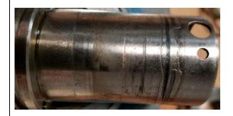
Gland worn on ID from contact with sleeve
