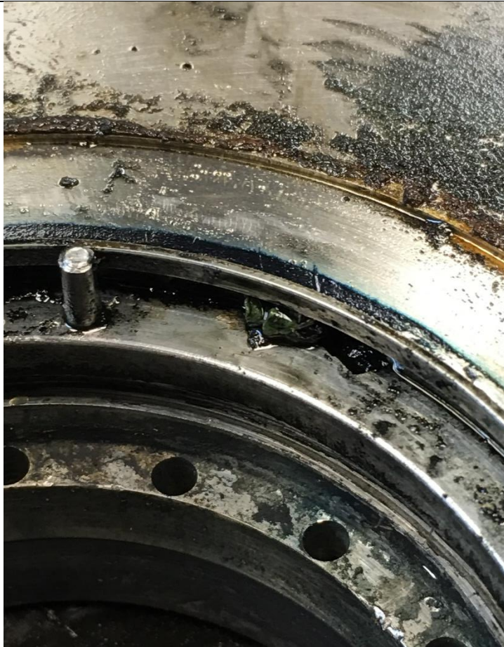
Figure 4: Hard debris found in flush port
