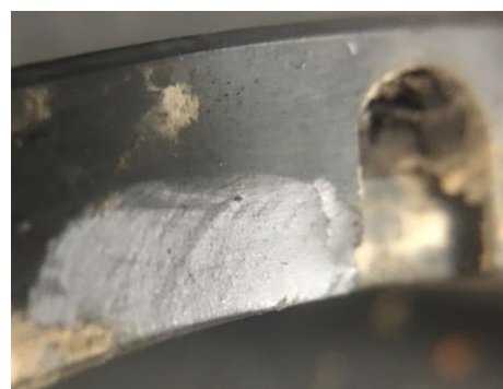
Figure 2: small chip by drive lug
