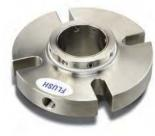
Premium-grade construction is standard, with options for FFKM or EPR elastomers and premium carbon, sintered silicon carbide faces. The FSI Series 1015 features viton elastomers, 316 stainless steel hardware. and a large flush port for API plan 11, 13, or 32 operation. Its self-aligning stationary design features a flexible stator that enables even face loading, and a four-bolt gland ensures the seal sets axially and radially.
